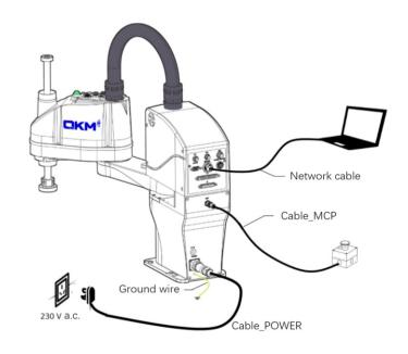
1. Install the network cable, ground wire, cable \_MCP and cable POWER according to the schematic diagram.
